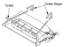
Figure 18 - Installing Grate (Pan Material Not Shown)
